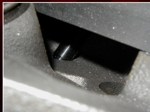
STEP 6: INSTALL THE APPROPRIATE STUD AND CHECK TO SEE THAT THERE IS FULL THREAD ENGAGEMENT INTO THE HEAD.
