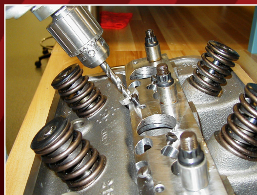
STEP 4: DRILL NEW HOLES FOR MOUNTING STUDS TO A DEPTH OF .870" \pm .025".
