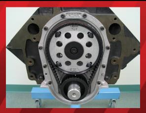
ROTATE CRANKSHAFT SO THAT TIMING DOTS ON CAMSHAFT AND CRANKSHAFT ARE ALIGNED.
