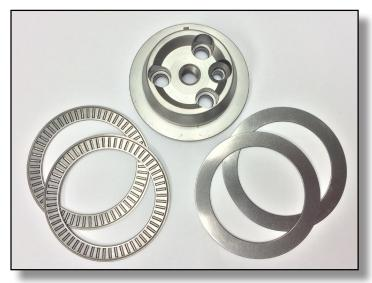
JESEL ZERO-THRUST CAM ADAPTER IS DESIGNED TO ELIMINATE LIFTER DAMAGING CAMSHAFT ENDPLAY. THIS ADAPTER IS MANUFACTURED FROM A HEAT TREATED TOOL STEEL AND IS SILVER IN COLOR. THE CYLINDER BLOCK MUST BE MACHINED TO RUN THIS ADAPTER. THE CAMSHAFT ENDPLAY CAN BE RUN AS TIGHT AT .001".
