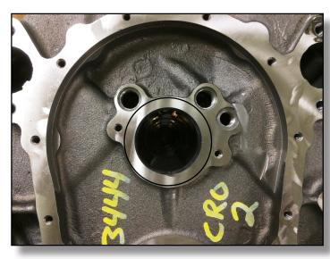
THE CAM TUNNEL MUST BE MACHINED 3.000" DIAMETER x .070" DEEP TO ACCEPT THE REAR TORRINGTON BEARING AND WASHER.
