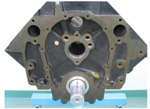
CHECK FOR COVER TO BLOCK INTERFERENCE AND CORRECT IF PRESENT BY MODIFYING THE BLOCK.
