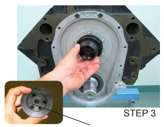
APPLY A VERY THIN LAYER OF RTV SEALER TO THE RECESSED AREA ON THE CAM ADAPTOR.
