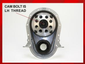
JESEL'S BELT DRIVE SYSTEMS ARE THE MOST ACCURATE AND DURABLE CAMSHAFT DRIVE SYSTEM AVAILABLE. A PATENTED HIGH TORQUE BELT OPERATES WITHOUT LUBRICATION AND SPINS WITH LESS FRICTION THAN CHAINS OR GEAR DRIVE SYSTEMS. THE BELT ALSO REDUCES THE AMOUNT HARMONICS TRANSFERED FROM THE CRANKSHAFT TO THE CAM RESULTING IN A SMOOTHER RUNNING VALVETRAIN. SOME FEATURES INCLUDE ABILLET ALUMINUM UPPER PULLEY, A HIGH TORQUE DRIVE BELT AND A HEAT TREATED ALLOY STEEL CRANK PULLEY.
