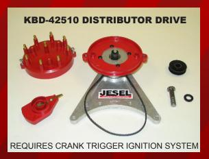
JESEL ALSO OFFERS A DISTRIBUTOR DRIVE KIT FOR THIS BELT DRIVE . THE DISTRIBUTOR DRIVE KIT ELIMINATES INACCURATE IGNITION TIMING SETTINGS DUE TO CAMSHAFT TORSIONAL TWISTING ON HIGH RPM ENGINES WITH EXCESSIVE SPRING PRESSURES. IT ALSO PROVIDES A MUCH COOLER LOCATION FOR THE DISTRIBUTOR. INTAKE MANIFOLD CHANGES WILL BE MUCH EASIER AS WELL THANKS TO THE DISTRIBUTOR NOT HAVING TO BE ROUTED THROUGH THE REAR PORTION OF THE INTAKE MANIFOLD. THIS KIT IS A DIRECT BOLT ON.
