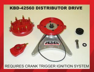
JESEL ALSO OFFERS A DISTRIBUTOR DRIVE KIT FOR THE BIG-BLOCK CHEVY. THE DISTRIBUTOR DRIVE KIT ELIMINATES INACCURATE IGNITION TIMING SETTINGS DUE TO CAMSHAFT TORSIONAL TWISTING ON HIGH RPM ENGINES WITH EXCESSIVE SPRING PRESSURES. IT ALSO PROVIDES A MUCH COOLER LOCATION FOR THE DISTRIBUTOR. INTAKE MANIFOLD CHANGES WILL BE MUCH EASIER AS WELL THANKS TO THE DISTRIBUTOR NOT HAVING TO BE ROUTED THROUGH THE REAR PORTION OF THE INTAKE MANIFOLD. THIS KIT IS A DIRECT BOLT ON.
